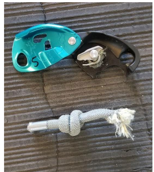
Figure 3. Ruptured Grigri ( U_{\text{force}}=9.7 kN) due to maximal slip (approx. 2m) to terminal knot with very worn, dry rope.
