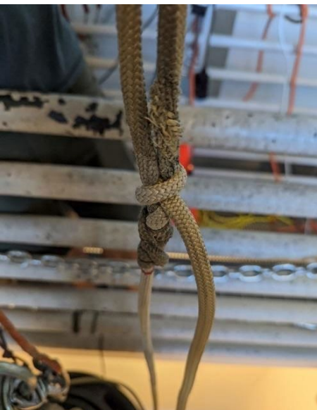
Figure 6. Clockwise from top left: damaged Rig (impact with terminal knot after maximal slip), rope severed by Safeguard, “slip and grip” pattern left on the rope after fall arrest by VT prusik, rope severed by Qrab, damage to VT prusik with 8 mm and 9.5 mm rope, respectively.
