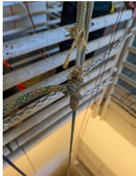
Figure 6. Clockwise from top left: damaged Rig (impact with terminal knot after maximal slip), rope severed by Safeguard, “slip and grip” pattern left on the rope after fall arrest by VT prusik, rope severed by Qrab, damage to VT prusik with 8 mm and 9.5 mm rope, respectively.
