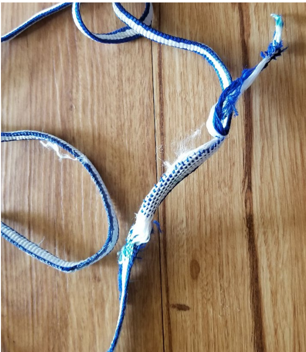
Figure 3: Sling damage via direct drop (test case 1).
