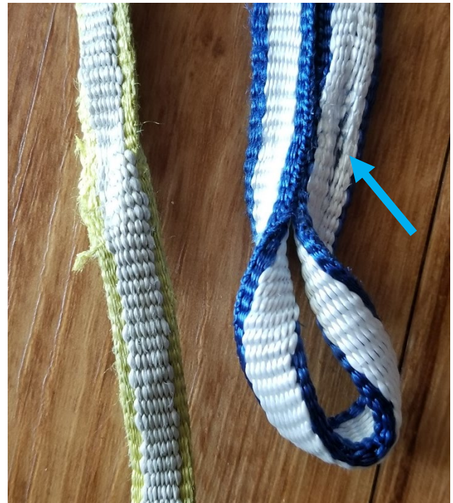
Figure 4: Sling damage from FF2 drops with dynamic rope (test case 2): abrasion (yellow), fusing and stretching (blue).
