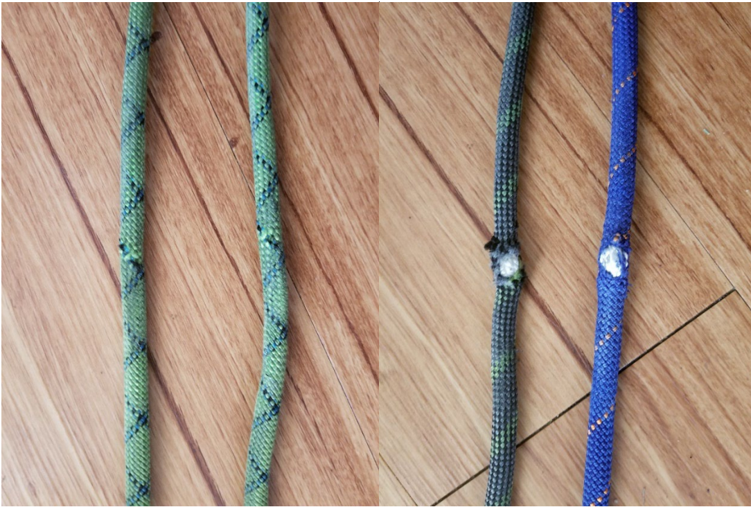
Figure 1: Representatives samples of rope damage—glazing (left) and core exposure (right).
