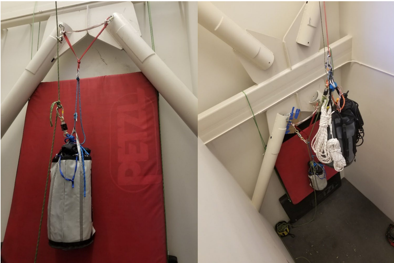
Figure 5: Test cases 1 and 2 set-up, belayer mass and anchor (left) and climber mass suspended from above (right).
