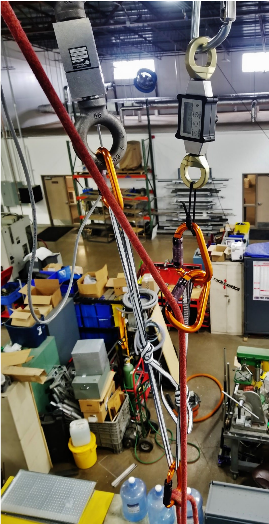
Figure 6: Detail of load cell with fuse and redirect carabiner.
