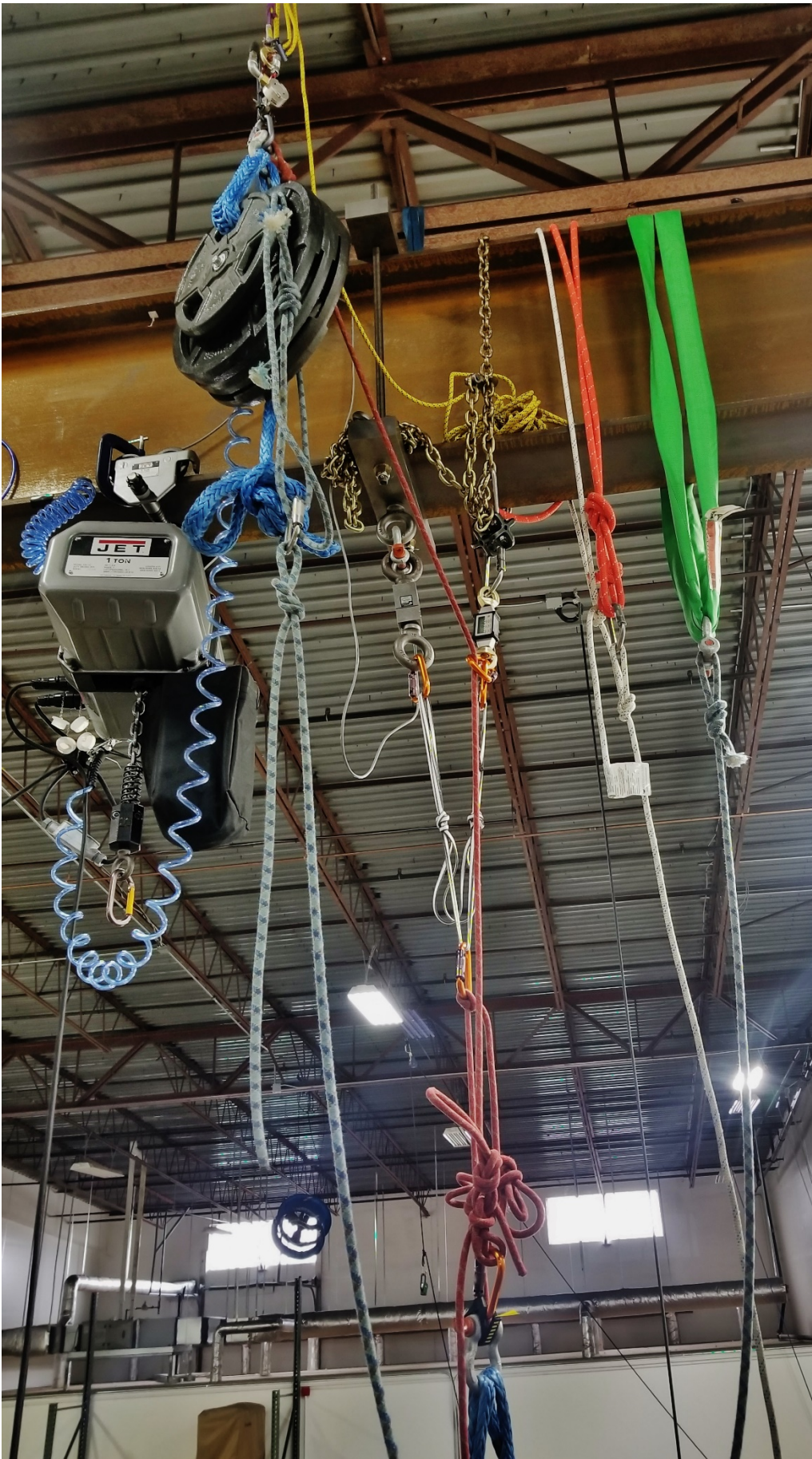
Figure 5: General rigging for test sets 1 and 3; differences vary between test sets. Test set 2 does not redirect the rope through the carabiner on the load cell with the fuse.
