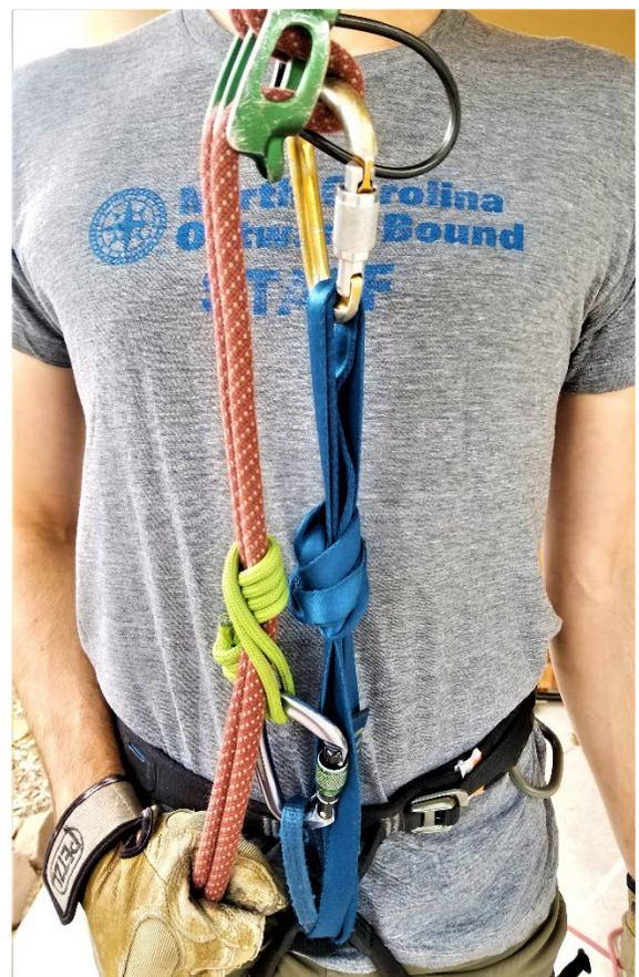
Figure 2. On the left, the friction hitch can be seen contacting the belay device upon inversion of the rappeller. To the right is an extended rappel, preventing the friction hitch from contacting the belay device even if inverted.
