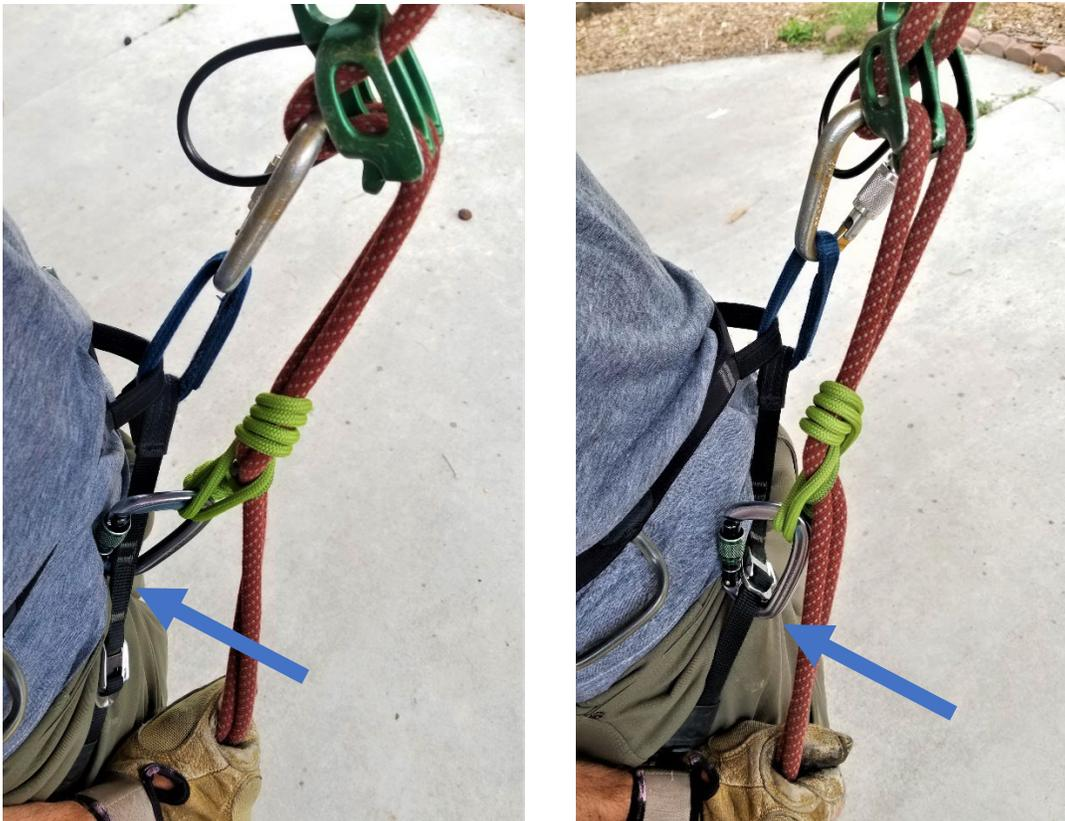
Figure 1. Note the carabiner affixed medially to (inside) the leg loop buckle in the photo on the left, and in the right photo, the carabiner affixed laterally to (outside) the buckle, pulling the buckle into the open position.
