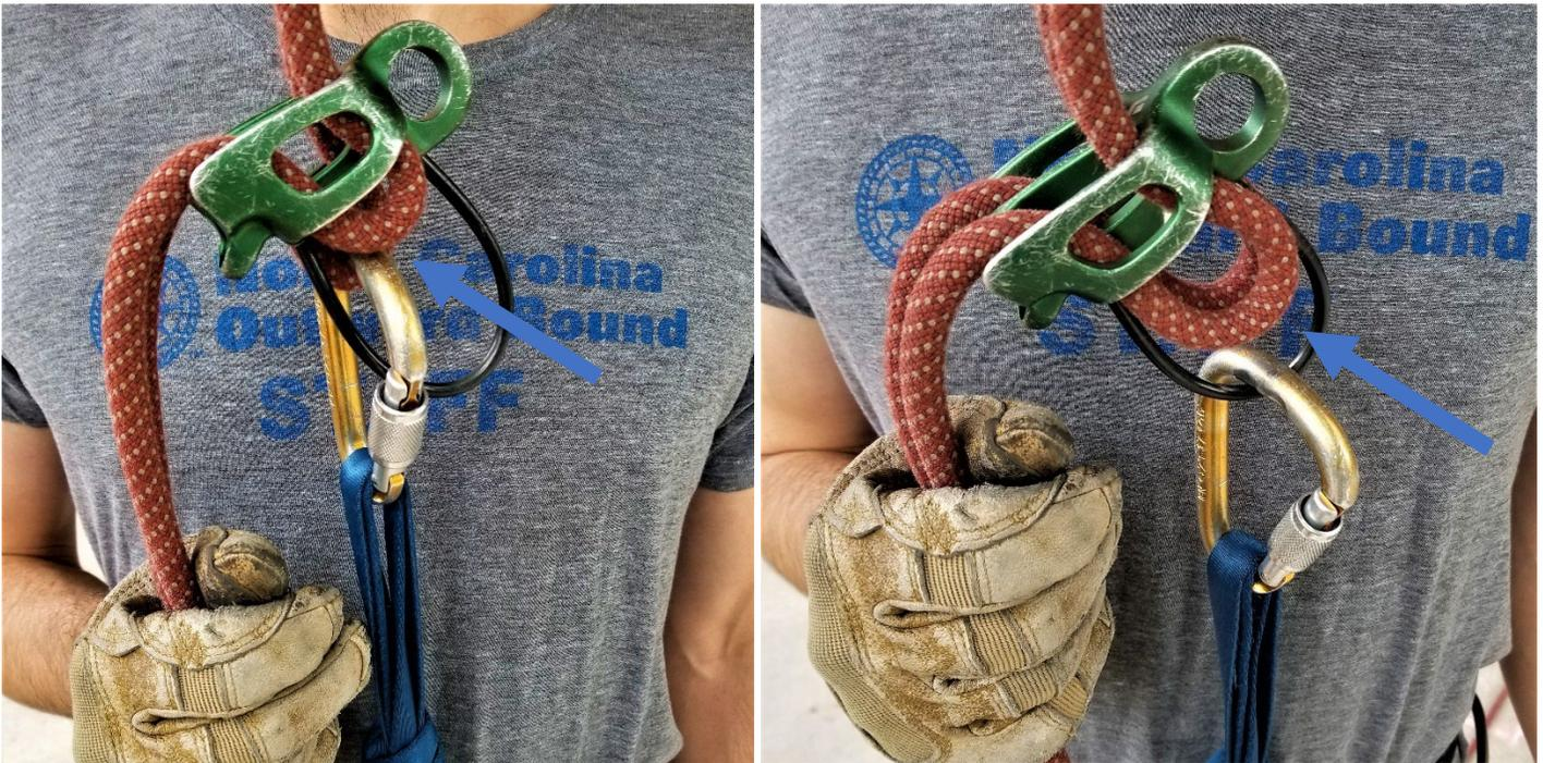
Figure 4. Mis-clipped rappel devices, with a single strand missed on the left, and both strands missed on the right.
